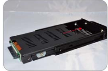
5. Push the cover of hard drive enclosure flatly to connect port.
