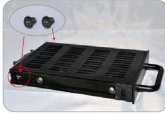
1. Take off the side screws of Hard Disk Drive.
