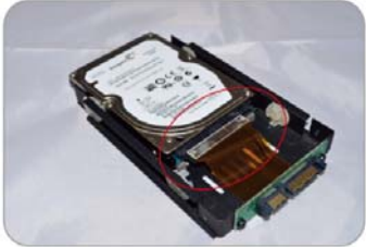
3. Connect the HD flat cable with 2.5”HD, make the alignment between HD & Shockproof plate and put the HD in.
