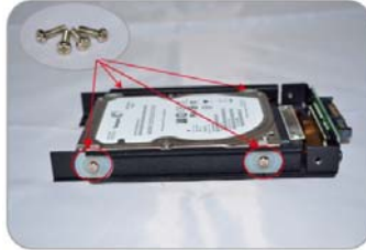
4. Lock four screws to fix the hard disk & Hard Drive Enclosure.
