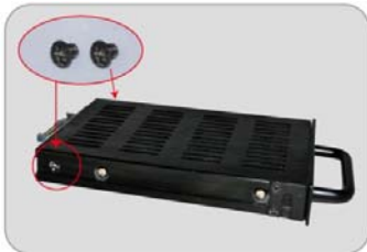
6. Lock two screws into both sides of hard drive enclosure.
