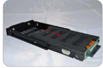
2. Push the hard disk drive connects port out in parallel.
