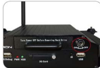
7. Install the hard drive enclosure into mobile DVR and make the lock of hard disk is on “ON” status.
